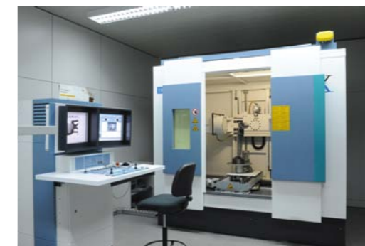
Internal control machine of aluminium structure with X-rays
