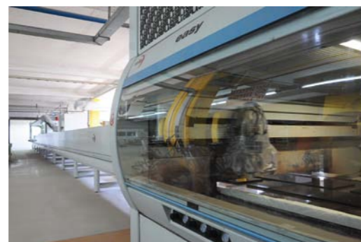
Painting and varnish of wooden surfaces
