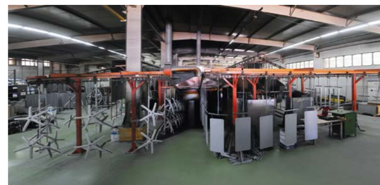
Complete system of electrostatic paint
